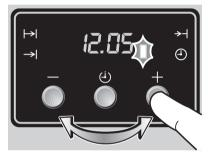
**3.** After approx. 5 seconds the function indicator will stop flashing and the clock will show the set time. The appliance is ready for use.
